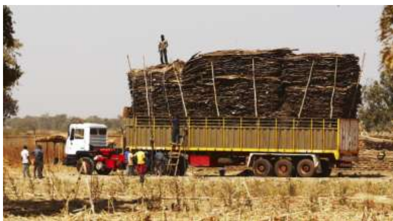
Figure 1: Overloaded truck lead to damaged roads which cost over $1 million per kilometer to replace
