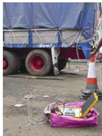
Figure 5: Portable weighbridge used by GHA at mobile weightstations
